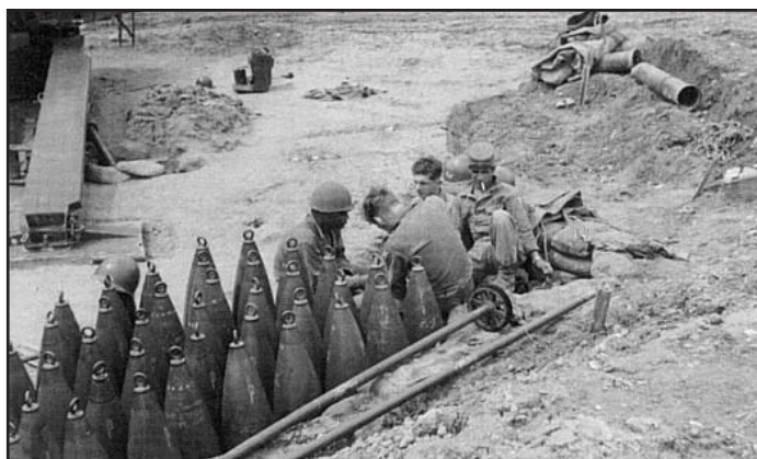
280mm projectiles (note the helmet on the second round from the left)
