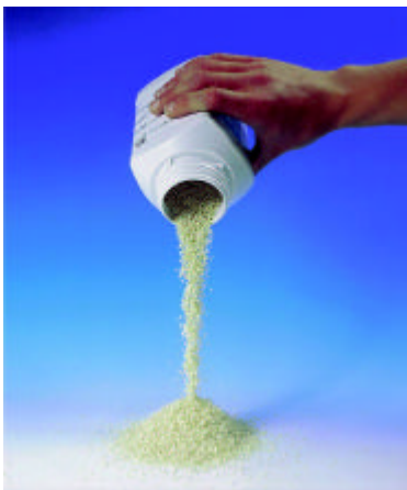
Figure: Merck's granulated dehydrated media (free flowing less dust, no clumping, dissolve easily and long shelf life)
