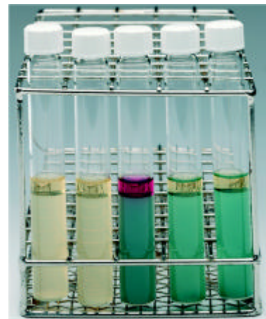
Figure: Fluorocult® LMX broth (left and right) Tube 1 and 2 S. enteritidis Tube 3 E. coli Tube 4 C. freundii Tube 5 Ent. cloacae
