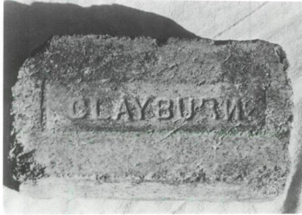
Fig. 7. A well-worn Clayburn firebrick, ca. 1905-09, pulled from an abandoned kiln in a rival brickyard in Port Moody, B.C. Note the backwards final "N" of "CLAYBURN" in the frog, an error which is not frequent in other Clayburn products of the era. (Photo by the author.)
