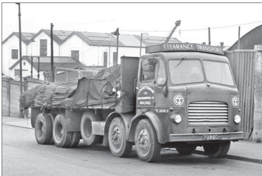
1962 Octopus 24.O/4 of Clearance Transport Ltd, Walsall where it was registered 709 BDH. Seen in Kimpton Road, Luton near Hayward Tyler's factory, Nov 1964. It appears to be equipped with tipping gear but is in use as a flat lorry here.
