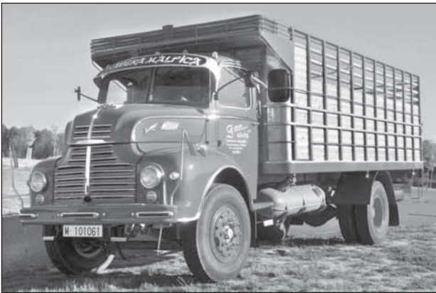
A typical Spanish body, with "domitorio" recessed into the front of the body
