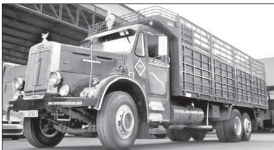
The Beaver with tag axle conversion by Jaufer
