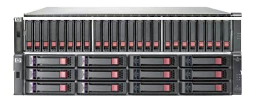
Delivers affordable, high-performing modular SAN arrays offering 8 Gb Fibre Channel, Combo Fibre Channel/iSCSI, 6 Gb SAS, 10GbE or 1 Gb iSCSI connectivity, 64 snapshots standard, and optional Remote Snap (replication) for Fibre Channel and iSCSI models.
