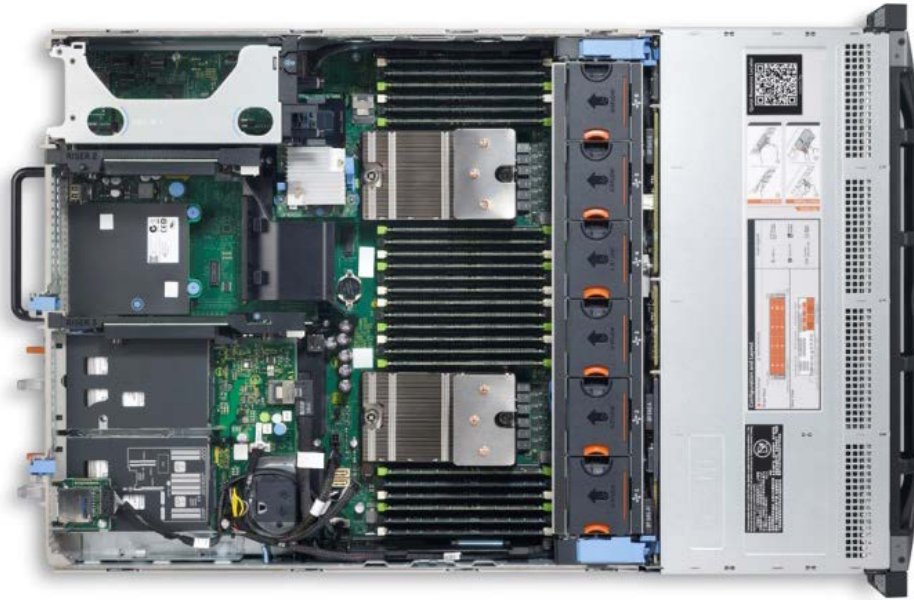
Figure 8. R720xd internal chassis view
