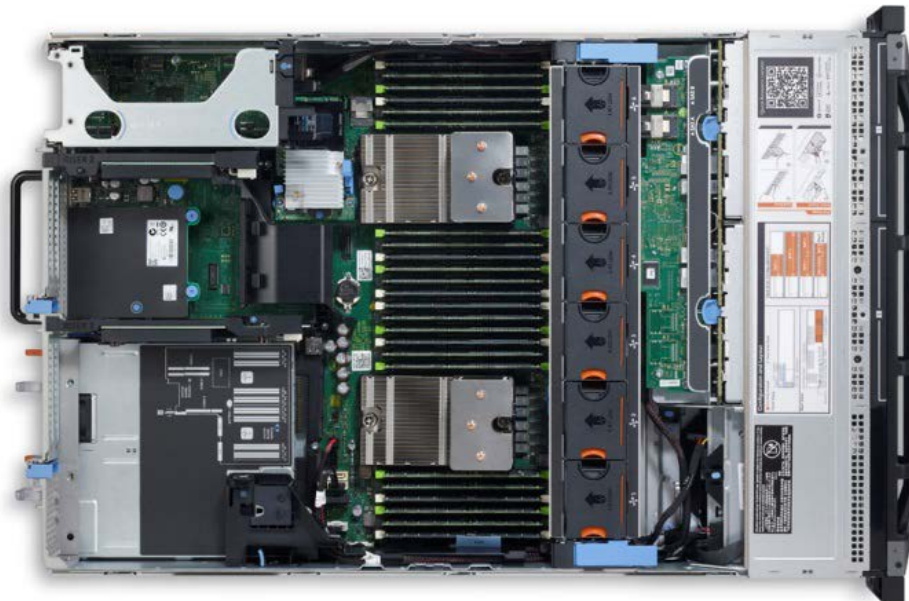
Figure 7. R720 internal chassis view
