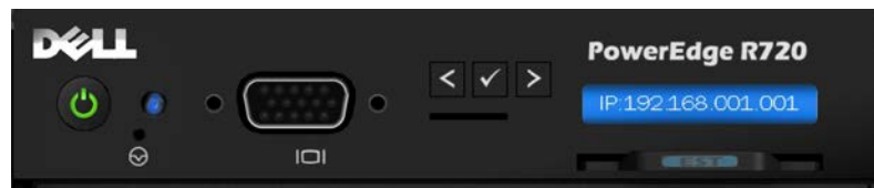
Figure 9. R720 LCD control panel
