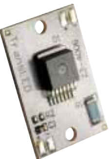
LED Strip DC/DC Driver 1 Driver per 6 modules maximum
