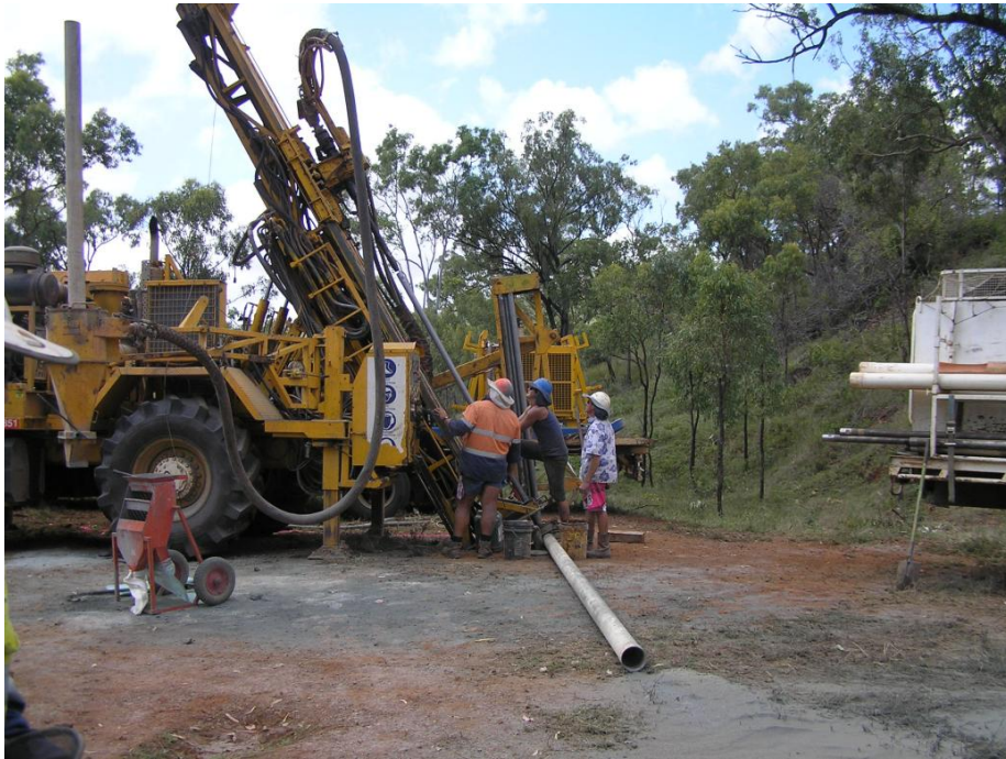
Figure 19 - Drill rig on site of IGRC002, looking south. Cyclone and sample splitter at left of photo (Terra Search, 2011).
