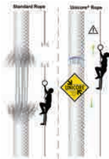
It allows escape if the sheath has been cut.
