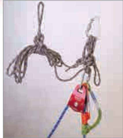
Tandem prusik belay set ups, when operated properly, are used to arrest or hold the load in lowering and raising systems.
