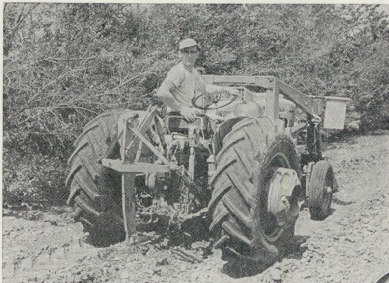
A subsoiling attachment for a farm tractor being used in the root-pruning of trees. Blade elevated. Note shoe at base of blade which leads blade into the ground. When lowered, the blade rides at an angle in the soil to a depth of approximately two feet.
