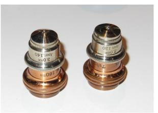
Figure 1 - Two ca. 1890's Zeiss high NA objectives
