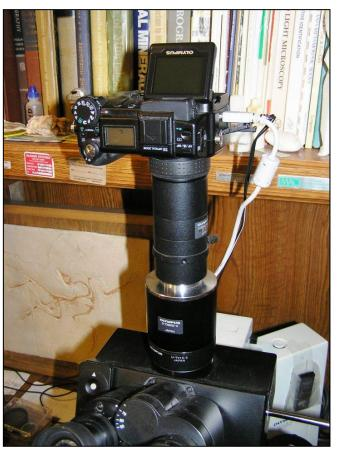
I like the C-5050 camera as it feels very solid and well designed. Olympus did a good job with making it work well on the microscope via the special adapter tube. The cameras are cheap enough now but the adapters are usually expensive, although once in a while a bargain appears on eBay.
