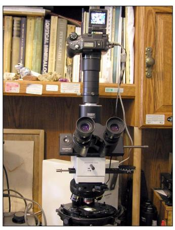
Figure 14 (left). The Olympus Camedia C-7070 at work on my BX50P microscope.
