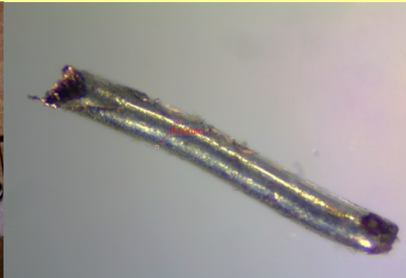
A very small piece of copper wire brightfield epi-illumination
