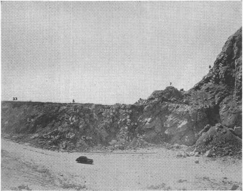
FIG. 7. South wall of Wet Weather quarry, September, 1940. Ls, limestone; Con, contact rock. Location numbers same as in Fig. 6.
