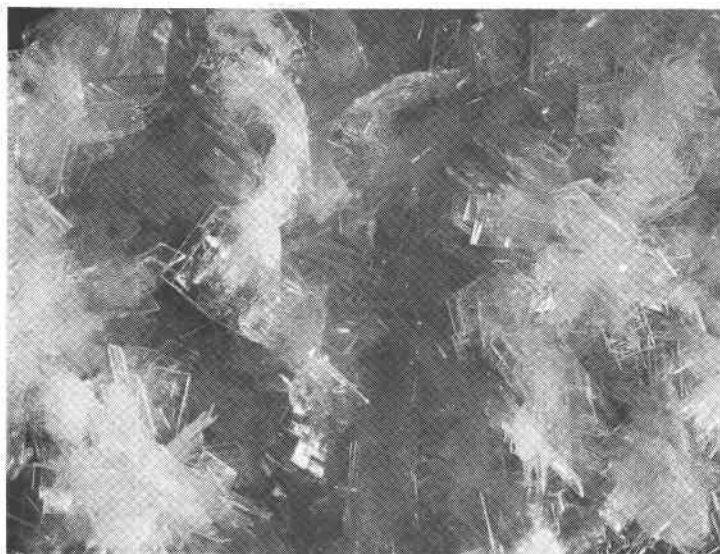
Fig. 2. Cluster of thin tabular synthetic crystals of darapskite. Magnification 10 \times .
