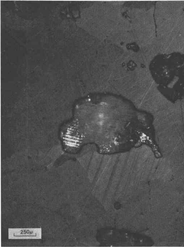
FIG. 1. Photomicrograph of paradocrasite showing polysynthetic twinning. Central area, showing internal reflection, is twinned calcite. Nicols partly crossed.
