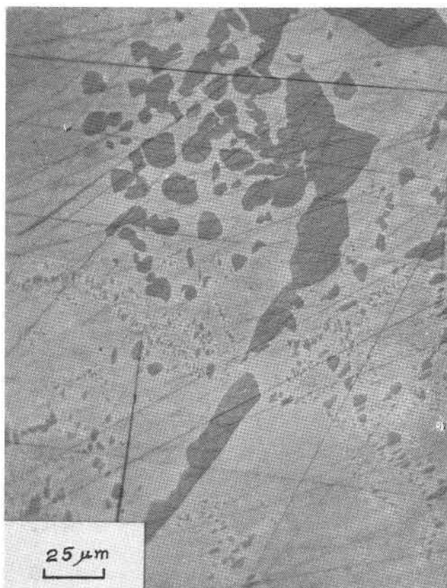
FIG. 4. Photomicrograph of exsolved blebs of stibarsen, the darker constituent, in paradocrasite. Contrast printing has exaggerated the distinction between host and guest and has produced bright halos about the smallest inclusions. Oil; green filter.
