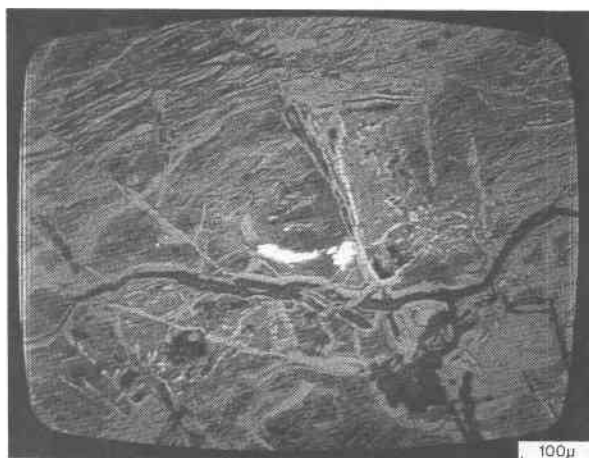
Fig. 2. Photograph of TV screen showing high-quality BE image at TV scanning rates. Polished section of gossan clearly shows a gold grain (bright); uncoated, 30kV.
