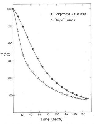
Fig. 2. Temperature-time plot comparing conventional compressed-air quench to that using the rapid-quench design. Each symbol represents an average of 3 values. Initial temperature was 600°C at a total pressure of 2.0 kbar.
