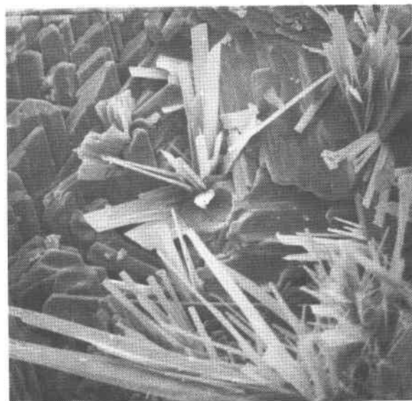
Fig. 3. Scanning electron photomicrograph of crystals of campigliaite grown on gypsum. Crystals are about 0.2 mm long.
