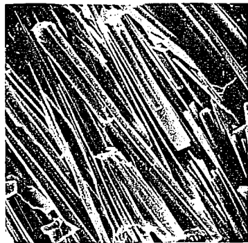
Fig. 2. Scanning electron photomicrograph of felted aggregates of lath-like, prismatic crystals of rynersonite (10,000X).
