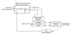
A remote command potentiometer provides the electrical signal for setting the speed of a hydrostatic drive. Moog Snap Trac electronics provide the necessary "black box" to complete the system. Various Snap Trac models are available for industrial use.
