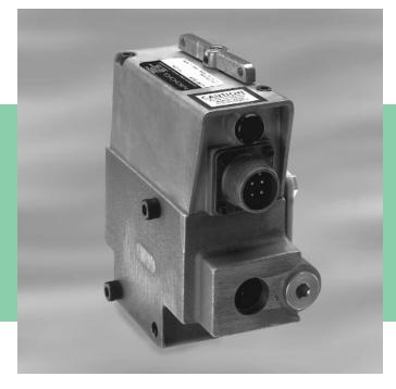
The Moog Controller provides electrical control of the swashplate angle, and so eliminates the need for mechanical interconnection between the operator and the pump. Instead, a simple potentiometer can be located near the operator with a pair of electrical wires running to the Controller. Alternatively, the Controller permits electronic control of the pump-motor combination. Electronic control makes numerous automatic operations
