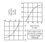
Typical Flow Characteristic - High Flow Controller
