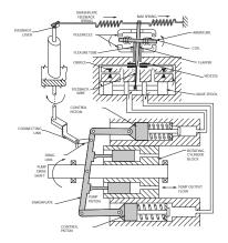
The Moog Controller\*, a replacement for the manual control lever and valve normally associated with hydrostatic drives, acts to position the swashplate in response to electrical commands.
