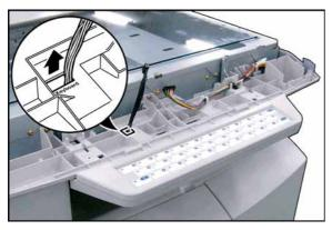
(14) Route the **Keyboard Harness** through the access hole on the machine.
