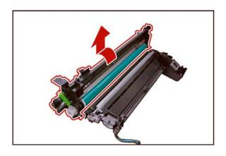
(12) Turn the **OPC Drum Assembly** in the direction of the arrow, and remove.
