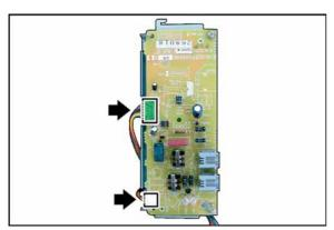
(22) Connect the **MJR Harness** to the MJR PC Board (CN22 and CN25).
