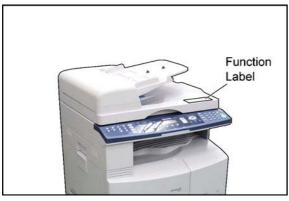
(32) Attach the **Function Label** (specified destination) on the upper right corner as illustrated.
