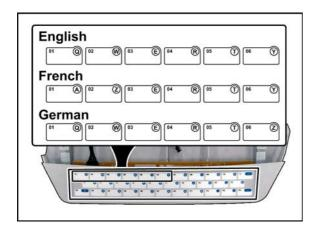
(13) Replace the preinstalled **Keyboard Sheet** to the desired language.
