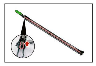
(28) Remove the Charge Wire Assembly.
