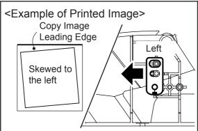
(B) If the Document is Skewed to the left, set the Adjusting Bracket to the left, and secure with 1 Screw.
