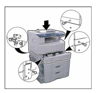
(34) Place the **machine** onto the 2nd Paper Tray Unit.
