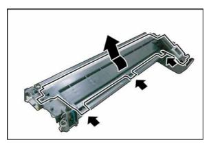
(13) Release 3 **Latch Hooks** and remove the **Developer Cover**.
