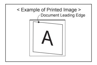
Adjust the Feed Skew Adjustment "A" downwards, and recheck the feeding alignment. Readjust as needed.
