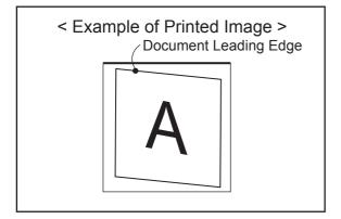
Adjust the Lever Plate downwards, and recheck the Document Skewing. Readjust as needed.
