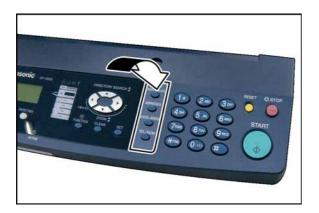
(12) Install the **Key Assembly** into the Control Panel Assembly.
