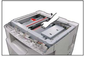
(5) Holding by the center, slowly move the **Lamp Base Assembly** to the center of the Scanner
