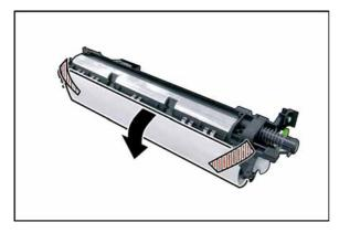
(24) Carefully remove the **Protective Sheet**, and **Tapes** from the OPC Drum Assembly.
