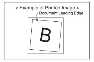
Adjust the Feed Skew Adjustment "B" downwards, and recheck the feeding alignment. Readjust as needed.
