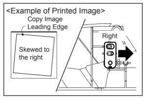
(A) If the Document is Skewed to the right, set the Adjusting Bracket to the right, and secure with 1 Screw.
