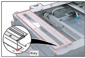
**Note:** When reinstalling the Left Document Plate, ensure the Scanning (S) Glass is in its original position against the key as illustrated.
