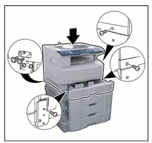
(54) Place the **machine** onto the 2nd Paper Tray Unit.
