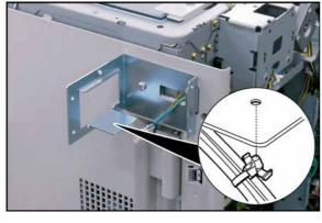
(33) Insert the **Harness Clamp** into the pre-drilled hole in the Key Counter Base (from underneath).
