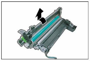
(12) Turn the **OPC Drum Assembly** in the direction of the arrow and remove.
