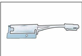
(60) Mount the **Dehumidifier Heater** onto the Dehumidifier Heater Bracket.
