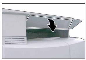
(11) Remove the Control Panel Sub Base Cover.
