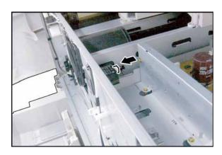
(19) Connect the **MC Harness** to the Mechanical Counter.
