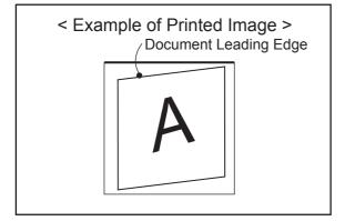
Adjust the Lever Plate upwards, and recheck the Document Skewing. Readjust as needed.
