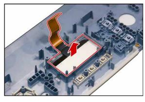
(25) Remove the  $\boldsymbol{LCD}$  Module (519).
