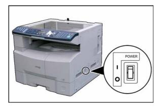
(31) Plug the **AC Power Cord**, and turn the Power Switch on the Right Side of the machine to the ON position.
