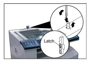
(1) Using a Slotted Blade Screwdriver, remove the **OPS Actuator** as illustrated.
