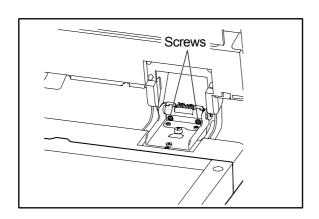
Fasten 2 Adjusting Screws on the Right Hinge. The Adjustment should be performed by 1/4 turn while checking the Free Stop.
