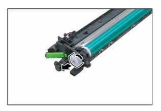
(13) Remove the **OPC Drum Shaft Holder** Assembly.
