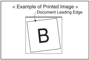
Adjust the Feed Skew Adjustment "B" upwards, and recheck the feeding alignment. Readjust as needed.
