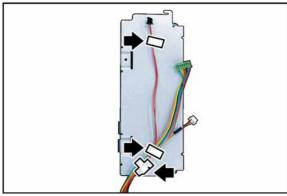
(21) Secure the **MJR Harness** with the Harness Clamps.
