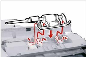
When reinstalling, make sure that the **Roller Holder** (2026) Assembly is properly placed on the ADF Unit.
