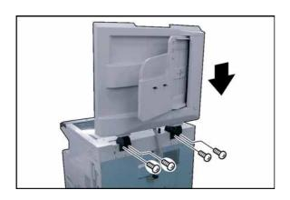
(1) Install the **Automatic Document Feeder** into the 2 Mounting Holes.
