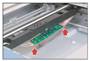
(8) Disconnect 2 **Harnesses** on the Inverter PC Board (CN1, and CN2).
