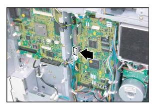
(25) Connect the KEY Harness to CN726 on the SPC PC Board.
