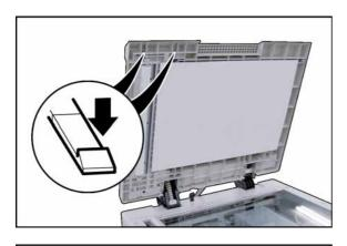
(20) Open the ADF, and release 2 Latch Hooks under the feeder.
