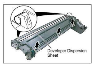
(16) Close the **Developer Cover**, and ensure that 5 Latch Hooks are hooked firmly.
