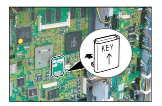
(3) Install the **Hardware Key** into the (CN67) connectors on the SC PC Board.
