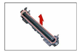
(26) Remove the Fuser Roller (1115) Assembly.
