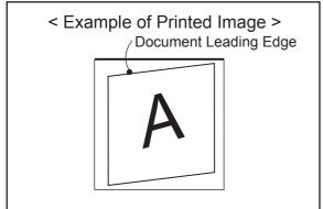
Adjust the Feed Skew Adjustment "A" upwards, and recheck the feeding alignment. Readjust as needed.
