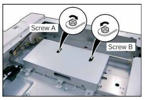
(4) Rotate the Screw A clockwise, and Screw B counter-clockwise by the same amount. (Half rotation of the screw, adjusts the skewed image by approximately 0.9 mm.)
