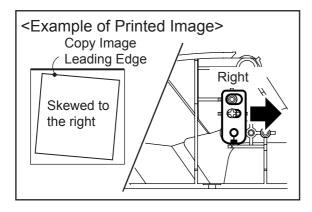
(23) If the Copy Image is Skewed to the right, set the Adjusting Bracket to the right and secure it with 1 Screw.
