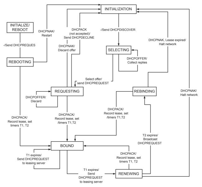
The client maintains two times, T1 and T2, that specify the times at which the client tries to extend its lease on its network address. T1 is the time at which the client enters the RENEWING state and attempts to contact the server that originally issued the client's network address. T2 is the time at which the client enters the REBINDING state and attempts to contact any server. T1 MUST be earlier than T2, which, in turn, MUST be earlier than the time at which the client's lease will expire.
