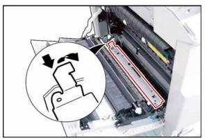
(9) Remove the **Pressure Plate** (649).
