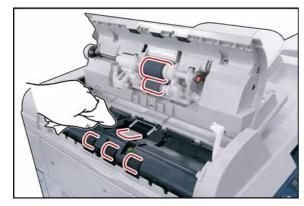
(3) Clean the **Separation Rubber**, **Feed Roller**, **Pre Feed Roller**, and **Paper Feed Roller** with a soft cloth, saturated with Water.
