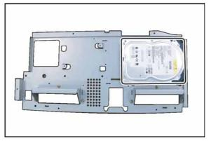
(19) Install the **HDD** into the Right Bracket as illustrated.
