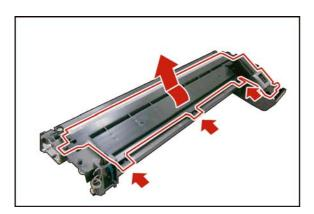
(13) Release 3 **Latch Hooks**, and remove the **Developer Cover**.
