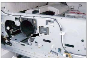
(18) Install the **Mechanical Counter** to the machine.
