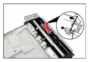
(49) Remove the **Timing Actuator** (2004).
