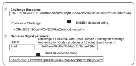
The authentication protocol exchange consists of a series of server challenges and client answers that are specific to the authentication mechanism. A server challenge, otherwise known as a ready response, is a 334 reply with the text part containing a BASE64 encoded string. The client answer consists of a line
