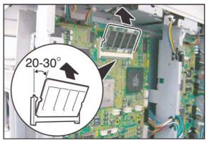
(3) Insert the **SDRM PC Board** into the Socket on the SC PC Board as illustrated.
