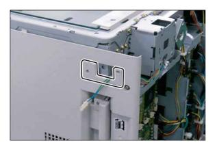
(30) Install the **Protective Tab** that was cut Step (28).
