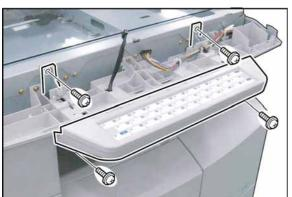
(16) Secure the Keyboard Unit with 4 Screws.
