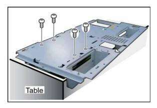
(20) Secure the HDD with 4 **Screws** (6-32x3/8).
