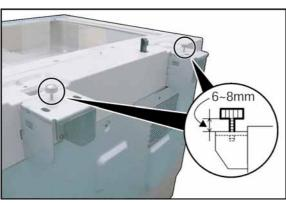
(5) Install 2 **Thumb Screws** (M4 x 10). (One for each ADF Mounting Bracket)
