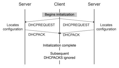
Timeline diagram of messages exchanged between DHCP client and servers when reusing a previously allocated network address
