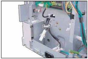
(58) Secure the **PTC-AC Harness 3** with the Harness Clamp.
