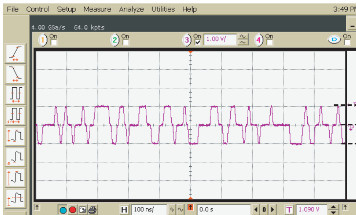
② 100Base-TX waveform 2 (A part of the waveform1 is magnified.)
