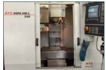
XYZ MINIMILL 560 with Siemens 810 CNC Control. Year 2005. Table 610 x 370mm. XYZ travel 560 x 400 x 500mm. Spindle taper BT40. Spindle Speed 8000rpm. Spindle Power 9.7kW. Rapid Feeds rates 20mm/min. ATC 20 Position. Coolant. Interlocked guards. Low Volt Light. Manuals.
