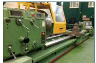
SWIFT 21D Heavy Duty CNC Lathe with Fanuc Oi-TD Control. Overhauled & retrofitted 2012. Swing over bed 42" 1068mm. Swing over saddle 30.5" 774mm. Maximum distance between centres 192" 4878mm. Maximum weight between centres (unsupported) 12 tons. Chuck dia. 41.5" 1054mm. Main spindle dia. 9" 228mm.
