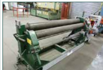
BUXTON 80" x 18" Initial Pinch Bending Rolls. Capacity 80" x 18". Motor 3kW.
