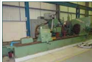
CHURCHILL TWA Roll Grinding Machine with Cambering Attachment. Travelling Wheelhead. Maximum swing 1,000mm x 3,000mm Between Centres. Face Width 5,000mm. Infinitely variable feeds. Maximum wheel diameter 750mm. Wheelhead speeds 420rpm/840rpm. Coolant/Filteration Unit.
