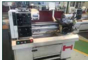
HARRISON M300 x 25" Gap Bed Centre Lathe. Swing Over Bed 13". Swing In Gap 16". Distance Between Centres 25". Travelling Wheelhead. Maximum swing 1,000mm x 3,000mm Between Centres. Spindle Bore 1.5". Spindle Speeds 40 to 2500 RPM. 3 Jaw Chuck. Quick Change Tool Post. Coolant.
