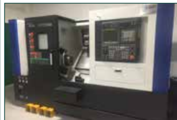
HYUNDAI Wia L230LMSA Slant Bed CNC Lathe with C Axis & Driven Tooling. Fanuc 32i. Year 2014. Main spindle Chuck dia. 210mm. Maximum swing 551mm. Turning dia. 305mm. Turning length 520mm. Spindle bore 77.97mm. Bar capacity 68mm. Main spindle 4.000 rpm. Main spindle nose A2-6. 20HP. Sub spindle nose A2-5.
