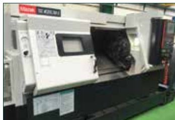
MAZAK Quick Turn Nexus 250-II CNC Lathe. Mazatrol Matrix Nexus Control. Year 2007. Swing over bed 610mm. Swing over carriage 350mm. Distance between centres 1000mm. Max machining length 950mm. X Axis travel 225mm. Z axis travel 1035mm. Spindle speeds 0-4000 rpm. Spindle nose A2-6. Spindle bore 87.5mm. Bar capacity 77mm. Turret 12 positions.
