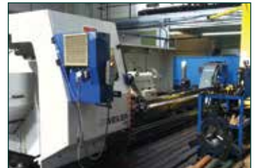
WEILER E90 CNC Oil Country Lathe with Ejector Drilling System. Siemens 940D Control. Year 2006. Swing over bed 900mm. Swing over cross slide 530mm. Distance between centres 4500mm. Twin Chuck dia 700mm. Spindle bore 62mm. Spindle speeds 1-700 rpm (2 ranges). Kopter 4 way manual tool post. Fused steady 40 - 300mm. Tailstock quill dia. 50mm.
