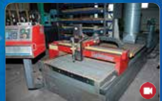
ESPRIT CNC LIGHTNING 1500 PROFILE PLASMA CUTTER + HYPER THERM HYDEF 3070 OR HPR130
