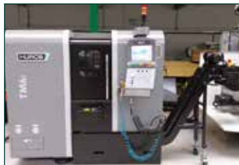
HURCO TM6I CNC Lathe with Multifed MV-65 Barfeed. Year 2015. max. cutting diameter (mm) 215. max. cutting length (mm) 318. Chuck diameter (mm) 152. Bar Capacity (mm) 45. X-Axis (mm) 170. Z-Axis (mm) 355. Feeds X/Z Axis (mm) 151/24. Spindle power 13 kW. Torque 113 Nm. Spindle speed 6000 rpm. No. of Turret stations 12.
