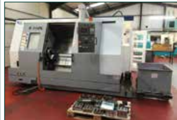
DOOSAN S550L 2 Axis CNC Slant Bed Lathe with Fanuc 21-TB CNC Control. Year 2005. Maximum swing 710mm. Maximum turning dia 550mm. Maximum turned length 1130mm. Spindle speeds 30-2500 rpm. Spindle power 22 kW. Spindle bore 102mm. Bar capacity 88mm. Rapid Feeds X & Z 20 & 26mm/minute. Tailstock taper 0MT. Tool setter. Coolant.
