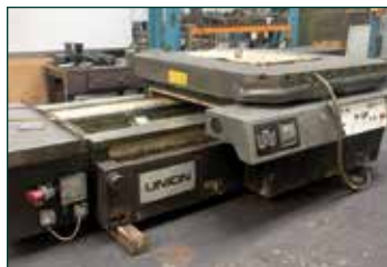
UNION TH1800 Powered Rotary Table. Table 1800mm x 2 000mm. Cross travel 1250mm. Loading 15 Ton. 9 kW. Volts 400V 3 ph 50 Hz. Weight 7.4 tons.
