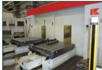
KURAKI KBM 11X-P Twin Pallet 5 Axis Horizontal Boring & Milling Machine with Fanuc 16-MB Control. Year 2003. Spindle dia. 110mm. Spindle speeds 5 - 3000 rpm. Spindle taper SK50. X/Y/Z/W 150/300/100/100 mm/25/50mm. Full B Axis indexing to 0.001". Rapids XYZ 12mm/min. Rapids W 6mm/min. 60 ATC. Table loading 2,200kgs. Main spindle drive (AC) 18kW.
