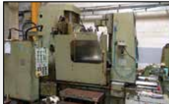
GEAR HOBGING STANKO YEAR 1999 CAP 1250MM
