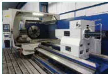
GURUTZPE A -1600 CNC Oil Country Lathe with 360mm dia. Spindle Bore. Twin Chucks & Fagor 8055 Control. Year 2008. Centre height 610 mm. Swing over bed 1,200 mm. Swing over cross slide 800 mm. Distance between centres 3,000 mm. Spindle speeds 0 - 480 rpm. Spindle bore 360 mm. Spindle nose A-20.
