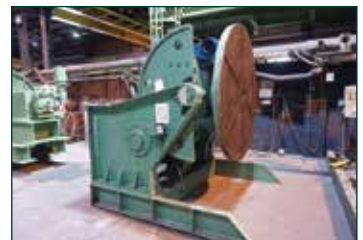
BODE Type ZVP/10 Welding Positioner. Power Table Tilting. Variable Speed Table Rotation. 10 Ton Capacity.
