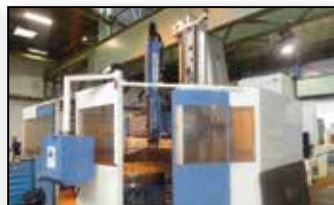
CNC VERTICAL TURNING BERTHIEZ TABLE 2000MM SWING 2800MM JOB HEIGHT 2000MM
