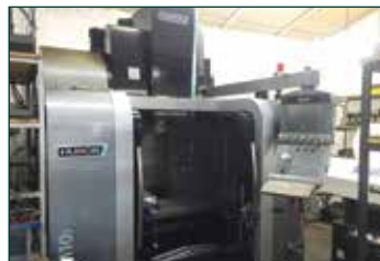
HURCO TM10I Vertical Machining Centre with WinMax Control. Year 2013. Table Size 762 x 366mm. Traverses XYZ 660 x 406 x 508mm. Spindle Speeds 10,000rpm. Spindle Motor Power 11kW. Tool Change Capacity 20 Station. Spindle taper BT40.
