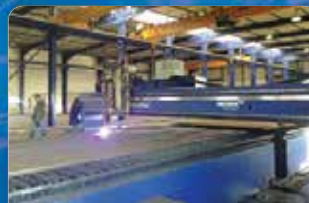
MESSER OMNIMAT 4000 CNC PLASMA & OXY FUEL CUTTING MACHINE Kjellberg HiFocus 360I and Extraction system
