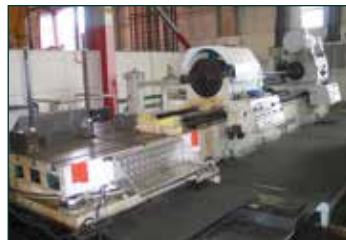
WOHLBERG B800P Heavy Duty Deep Hole Borer & Trepanning Machine. The "P" version is suitable for boring heavy, asymmetrical or awkwardly shaped workpieces, which cannot rotate. Workpieces of this type are clamped to a T-slotted indexing work table which has the capability of indexing 360 degrees in 4 x 90 degree graduations.
