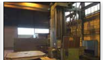
FLOOR TYPE BORING SCHIESS FRORIEP SPD 150MM DIGITAL TRAVELS 7000X3700MM SKODA TABLE 2000X2000MM
