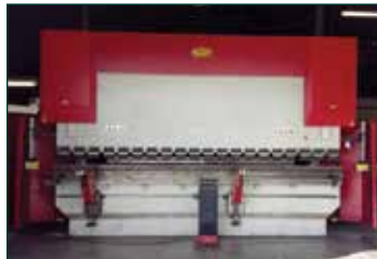
MORGAN RUSHWORTH PBXS CNC 4100/300 Hydraulic Downdroking Pressbrake. Year 2014. Capacity 4100mm x 300 Tons. maximum stroke 320mm. ESA S560 Touch screen controller. Fiesler Elektronik Akas-LC II safety light guards. Machine hours 1105. Tooling.
