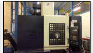
VMC MAKINO V 55 YEAR 2000 FANUC 14000RPM TRAVELS 900X500MM
