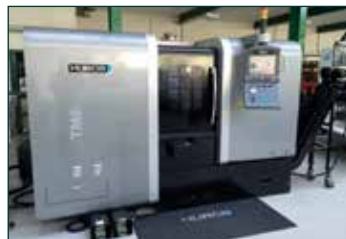
HURCO TM8I CNC Lathe with Hydrafeed MV65 Barfeed. MAX CNC Control. Year 2013. Max. cutting diameter 256 mm. Max. cutting length 458 mm. Chuck diameter 203 mm. Bar Capacity 52mm. X-Axis 203 mm. Z-Axis 508mm. Feeds XYZ 19/24 mm. Spindle-motor 16 kW. Torque 180 Nm. Spindle speed 0-4800 rpm.
