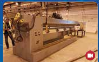
ESAB ID INTERNAL SEAM WELDER MODEL ID50 For Vessel, Cylinders & Tanks. SubArc or Plasma welding
