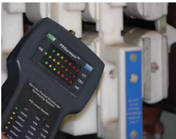
PDSurveyor™ testing AIS for Surface PD
