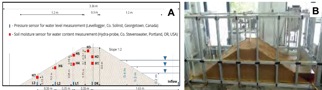
108 Figure 1. Sketch of the experimental setup including the positions of soil moisture sensors and pressure head sensors (A) 109 and picture of the dike experiment exemplary with 20 cm flooding (B)
