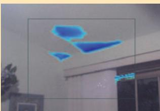
**IR/color alarm:** Isolates problematic areas by displaying a visual image with infrared highlights for surface temperatures in between, above or below, or outside a user-selected range.
