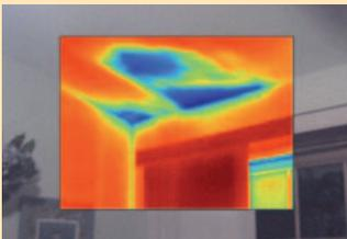
**Picture-in-picture:** Maintains a frame of reference by placing an IR "window" within a visual (visible light) image.
