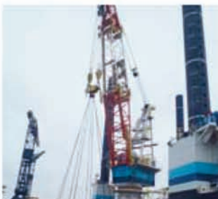
Offshore Crane FAVCO PC 1000 for Jack Up Barge B.V Lifting capacity: Max. Lift 1000 tonne @ 22m radius Boom Length: 60.76m to 97.23m
