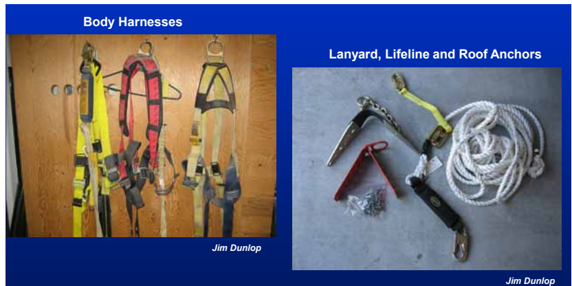
Figure 87. A personal fall arrest system (PFAS) consists of an anchorage and connectors, a body harness, and a lanyard/deceleration device.
