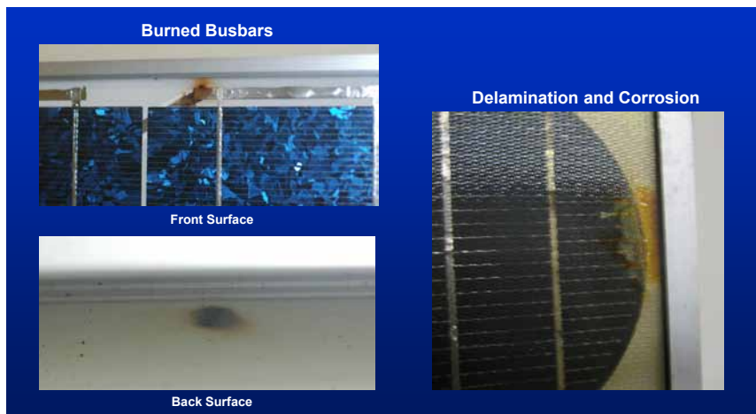
Figure 110. PV modules should be carefully inspected for any signs of discoloration, corrosion or delamination.
