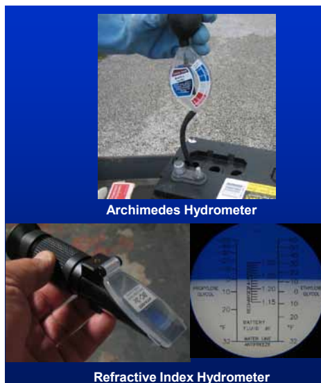
Figure 117. Hydrometers measure electrolyte specific gravity (SG).
