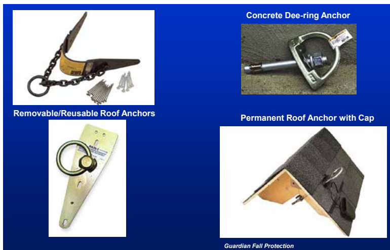
Figure 88. Safety line anchorages must be independent of any platform anchorage and capable of supporting at least 5,000 pounds per worker.
