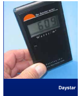
Figure 112. Handheld solar meters use a small PV cell to measure solar irradiance.
