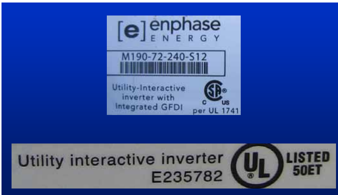
Figure 99. Inverters and ac modules used in utility-interactive PV systems must be listed and identified for interactive operations.
