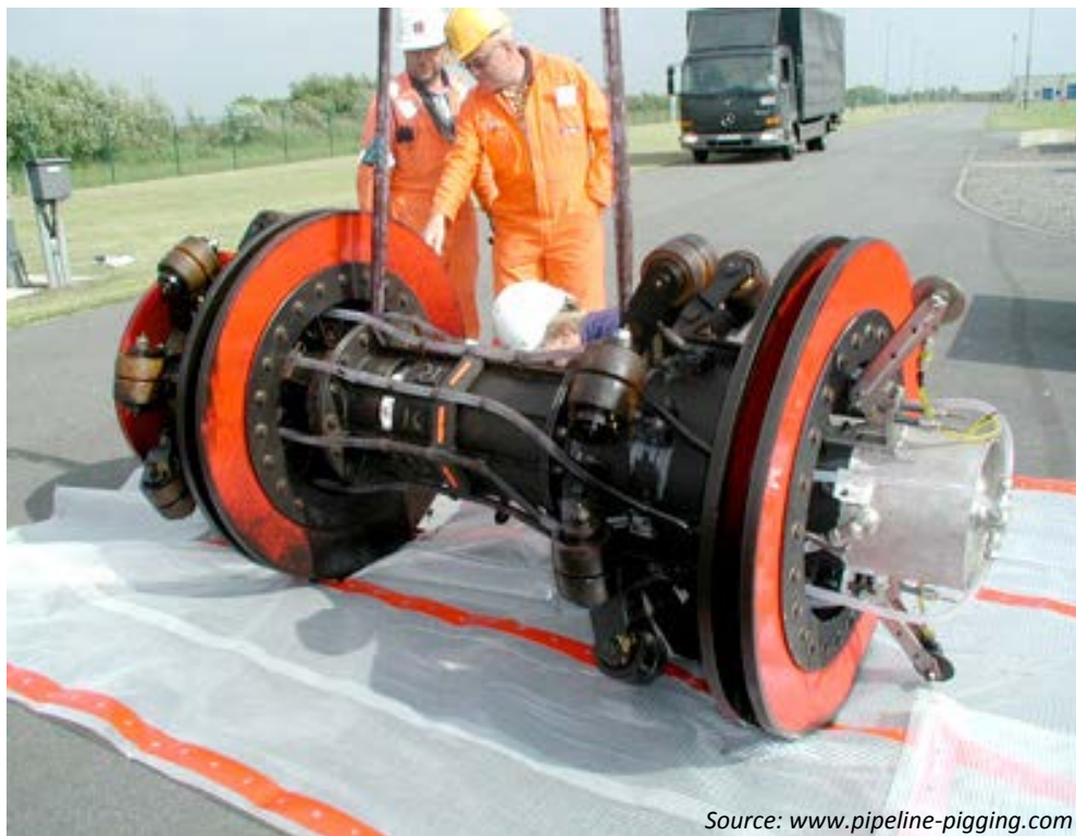
FIGURE 3-2: EXAMPLE OF A CLEANING PLUG, “PIGS”
