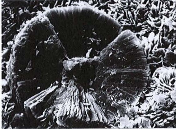
Fig. 2. Back-scattered SEM images of dypingite from Dypingdal, Snarum. Recorded at Mineralogisches Institut, Universität Karlsruhe in 1980. Images a, b and c show the globular form of the mineral; image d is an enlargement of the globule surface. The two lower images e and f show broken globules, revealing scaly texture and hollow centres. Width of images: a 0.6 mm, b and c 0.35 mm, d not recorded. The diameter of the globules in e and f is 0.13 mm.
