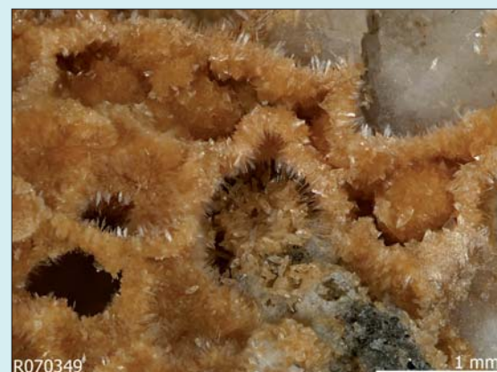
Figure 4. Chiavennite, \text{CaMn}^{2+}(\text{BeOH})_2\text{Si}_5\text{O}_{13} \cdot 2\text{H}_2\text{O} , in aggregate of pale yellow to orange spearhead-shaped blades associated with orthoclase and analcime from Tvedalen, Larvik, Vestfold, Norway. Photograph of sample R070349 reproduced with permission from the RRUFF Project (Downs 2006).
