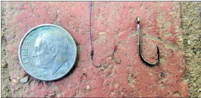
Figure 1. From left to right Gamakatsu Ultimate Tanago Hook, Owner Smallest Hook, and an Eagle Claw size 8 Bait-holder hook for comparison.
