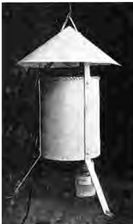
Fig. 11.—Light trap. (Photograph by courtesy of Bureau of Entomology and Plant Quarantine, U.S.D.A.)
