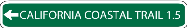
Supplemental plaques may be used in conjunction with the "Bike Route" sign
