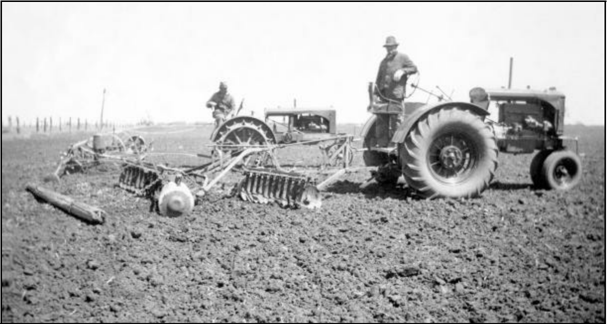
Figure 7.33 Seed bed preparation and planting with a disk and drag in the foreground, corn planter in the background. (5-18-1938)
