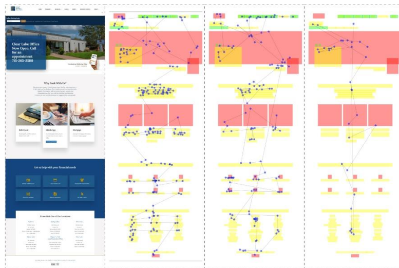
Fig. 2 Visualizations of gaze paths for three participants, overlaid on different web primitives: images (red), texts (yellow), and functional UI elements (green). The last participant (far right) appears to have explored the webpage superficially, with only a few fixations.
