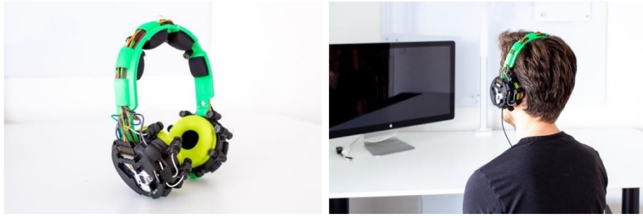
Fig. 2. Dry-electrode wearable EEG system for cognitive load monitoring (see [18]).
