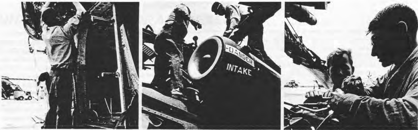
MAINTENANCE KNOW-HOW —In first photo, ADAN Billy Conley works on engine of one of HC-5's "Super Charlie's." In second photo, two maintenance crewmen from the squadron check the rotor on another UH-2C. In third photo, AD2 Carlos Chamberlain, left, and AD3 John King install a transmission oil tank line on one of the twin-engine helicopters. (USN photos by JOC John J. Gravat, PacFlt Combat Camera Gp)
