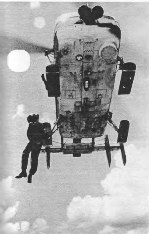
PRACTICE PICKUP —At left, a forest penetrator seat is utilized to hoist a crewman to an HH-43 during one of the numerous practice sessions held by Det 3.
