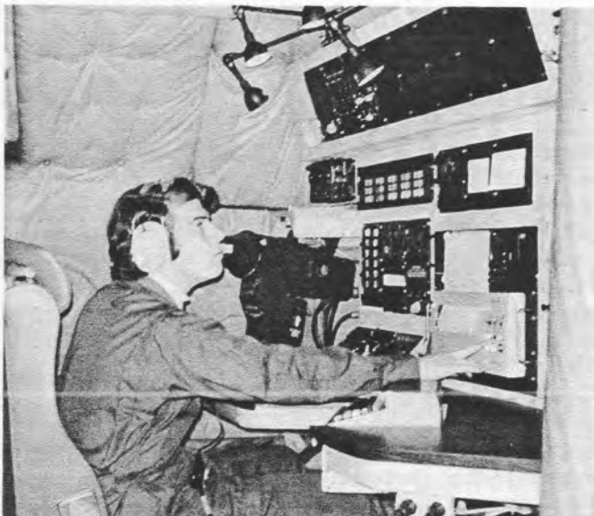
Robert Gilchrist checked out portions of the airborne weather reconnaissance officer's (ARWO's) equipment. The ARWO, or meteorology officer, is the mission controller on weather reconnaissance flights. All key data is channeled through his equipment for display, recording and analysis.
