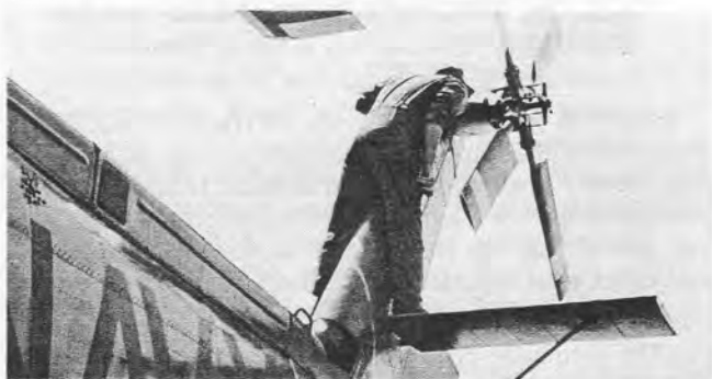
AMS3 Terry Goodpaster inspects tail rotor gearbox.
