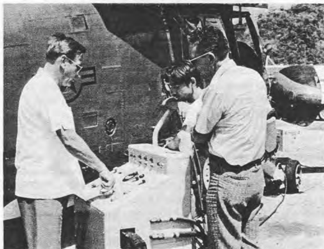
AX2 Steven D. Powers, middle, and KAC rep Donald Lockridge watch as Donald Delaney, also a Kaman rep, operates controls on hydraulic test stand.
