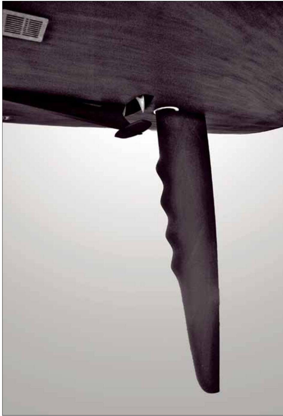
Paul Bieker employed tubercles, shown above, on the rudder design to provide extra control in challenging conditions. Below, the engineering of the retracting drive unit is simple and effective.
