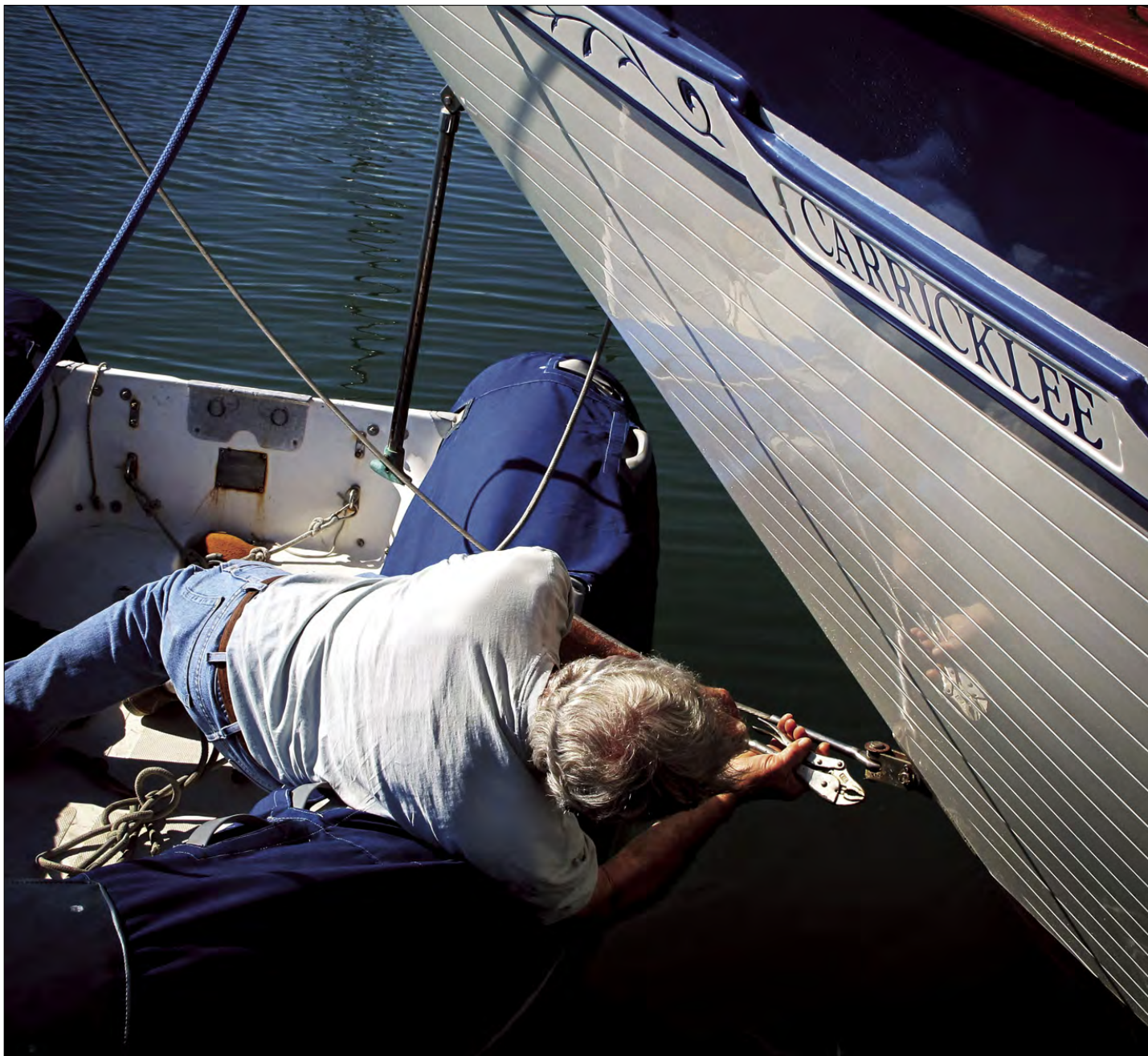
Bob installs a newly fabricated bobstay to replace the back-up spare he installed at Isla de San Cristóbal, Galápagos.
