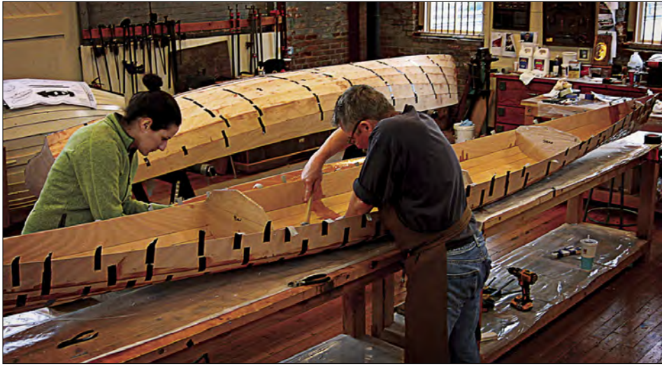
Angela Cosby (Astoria Parks and Recreation director) and instructor Chuck Bollong work on fiberglassing the interior keel joint of her 17' Pygmy Murrelet kayak.
