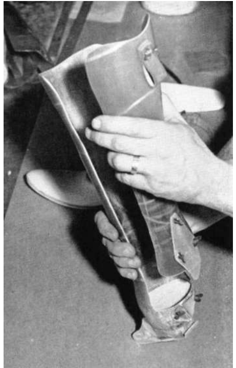
Fig. 21. Tongue-and-slot method of holding corset in place. Tongue and slot are held in place temporarily by the bolts and wing nuts. Epoxy resin and rivets are used for permanent attachment.
