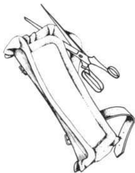
Fig. 43. Final step in fabrication of cover for opening in side of socket.
