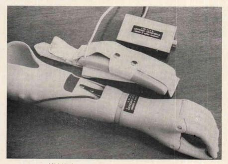
I.N.A.I.L. System: Prosthesis, battery pack, and amplifier
