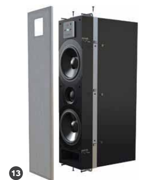
13 Storm Bluetooth Speaker • STORM is a premium quality sound system that is designed specifically for furniture integration including wine racks, kitchen islands, 150mm cupboards and side panels • Speaker unit: H:405 W:112 D:200mm • Fascia: H:425 W:120 D:5mm • Designed for flush or recessed installation • 80W music power per unit • Actisonic patented sound technology 144023
