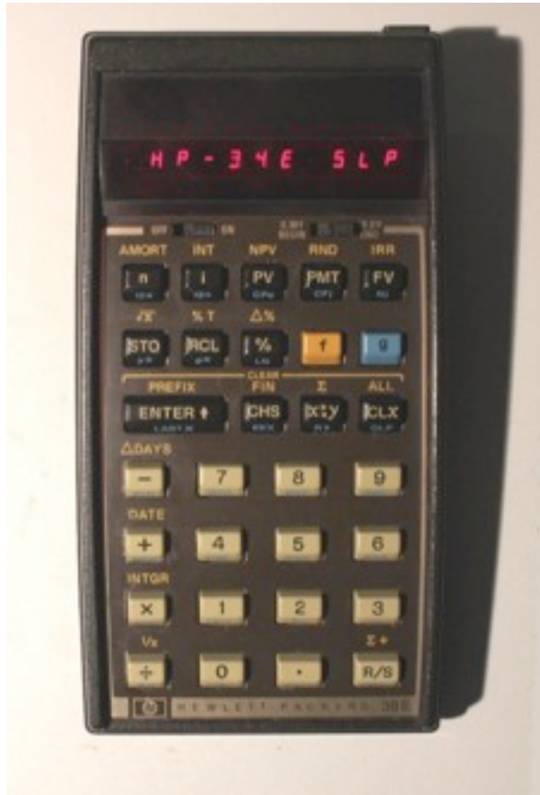
HP-38E converted to Multi SPICE calculator HP-34 SLP including HP-31E/32E/33C/34C/37E/38C
