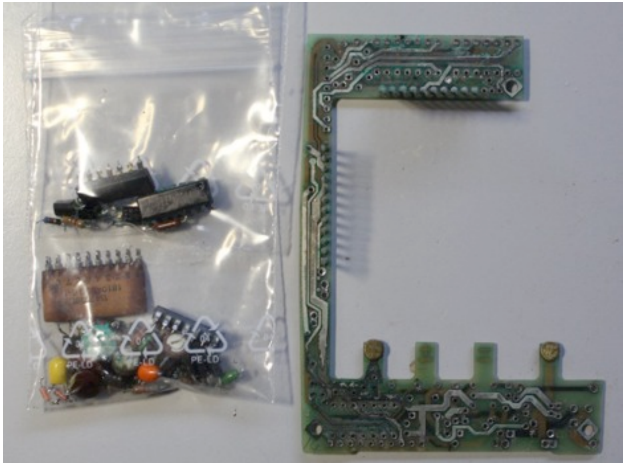
HP-19C power supply/printer board, all components removed
