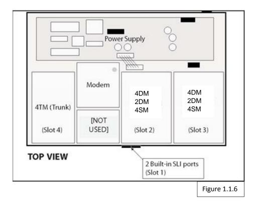
The base cabinet has openings for mounting the cards into the cabinet. When the cards are mounted, the RJ45 connectors provide an interface to 4 CO lines, 8 extensions, 2 single line
