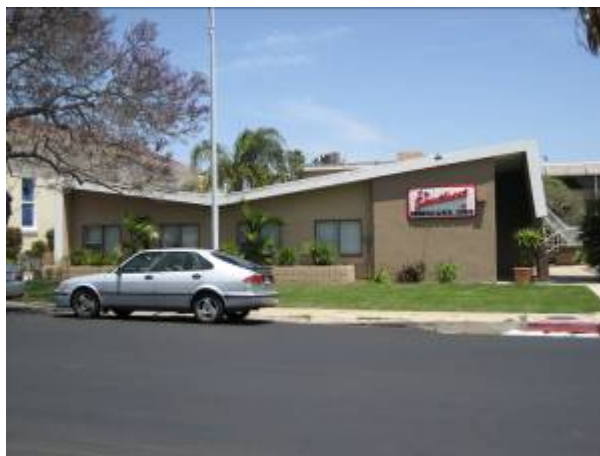
Office building in Point Loma, designed by Richard Wheeler. Note the butterfly roof line and sunshades at the eave.
