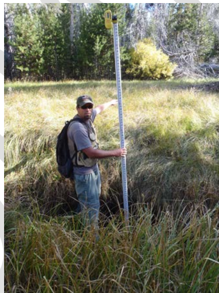
Photo 4: Incised channel (North Fork of Angora) no longer connected to meadow floodplain (arm level)
