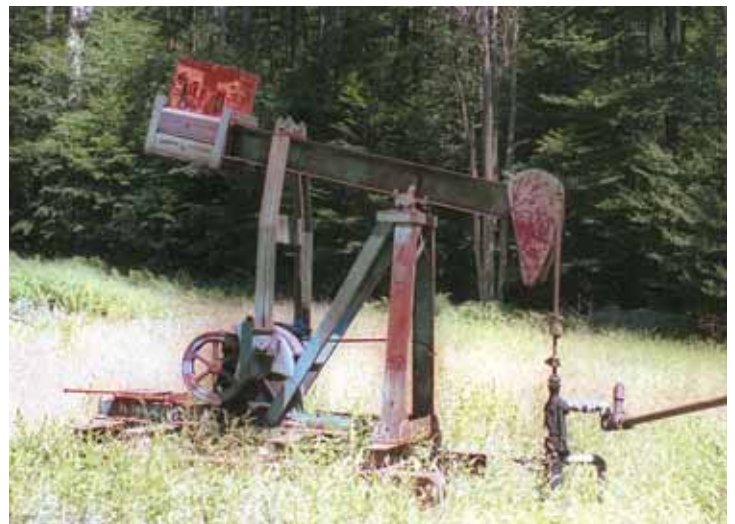
Typical pumpjack found in the Allegheny National Forest. Since the late 1800s, tens of thousands of oil and gas wells have been drilled in the region to help supply the nation’s energy demands.
